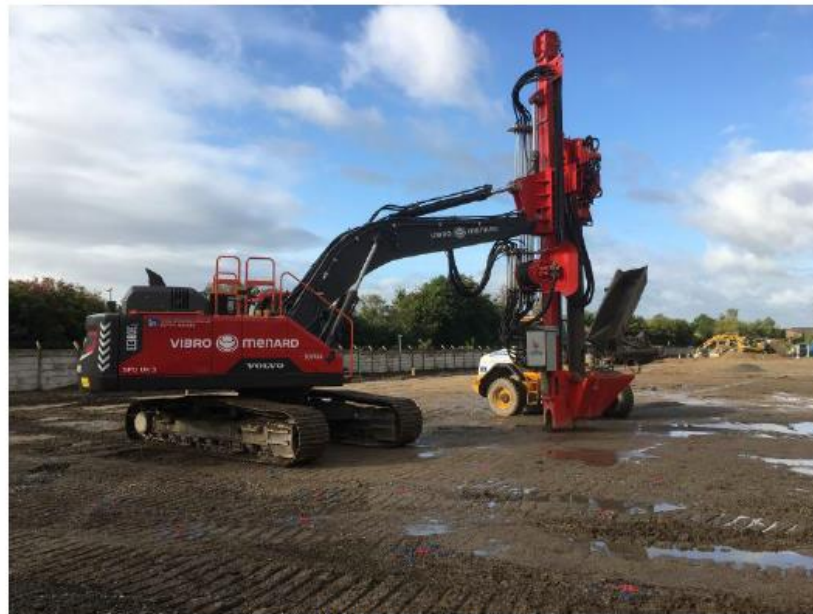
Figure 3 – VSC rig on site
